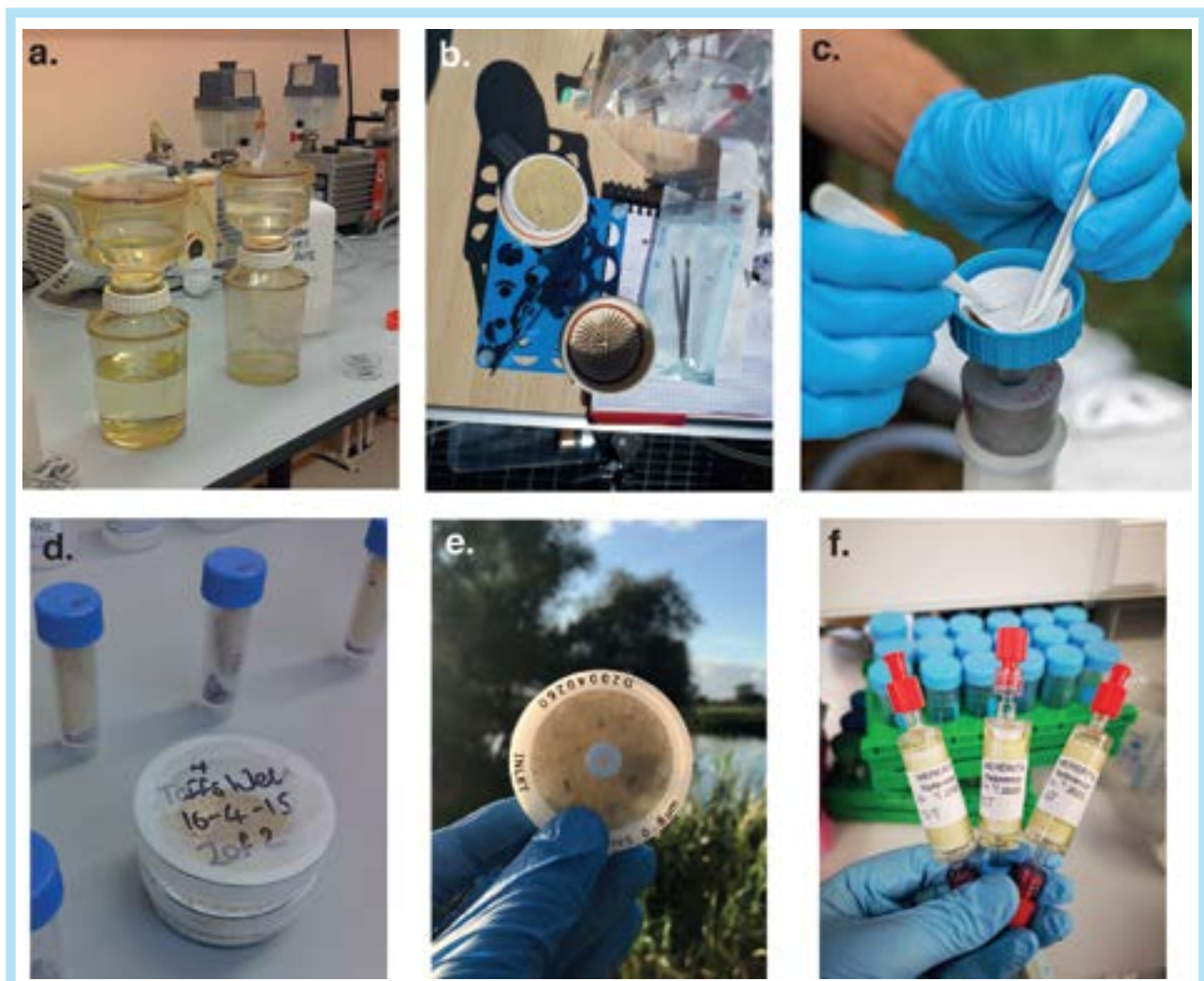
Figure 3. Water eDNA filter types. 1: Open filters are exposed to the air during filtration either in the field or lab (a and b). 2: Housed filters are a membrane placed in a solid unit during filtration (c). Filters from Open and Housed units need to be removed from the filtration unit and stored in a petri dish or eppendorf tube until extraction (c and d). 3: Enclosed filters are systems in which the membrane is enclosed within the outer housing (e and f). Extraction is carried out directly from the enclosed filtration unit.
